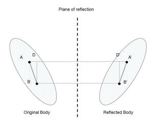
Figure 2: Geometry of Planar Rigid Body Reflection
