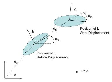
Figure 1: Geometry of planar displacement
