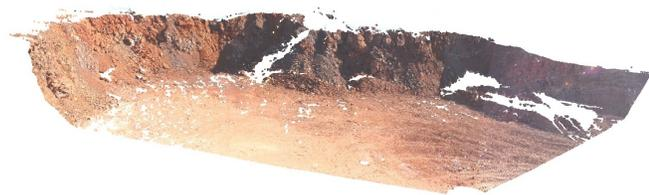
Fig. 3. Laser Scanner data set taken at Mt. Tom Price mine in Western Australia using a RIEGL LMSZ420. The data set consists of over 1.85 million data points. The data set spanned about  $135 \times 72$  sqm.
