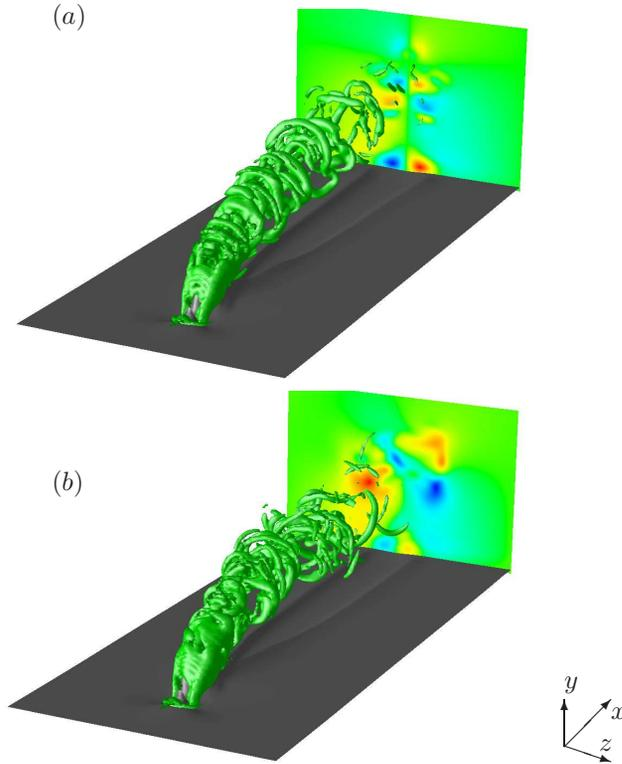
FIGURE 1. Instantaneous snapshots of cases (a) DNS-SYM and (b) DNS-ASYM at  $t = 700$ . The vortical structures are visualized by means of iso-contours of constant  $\lambda_2 = -0.09$  (green); the gray contour depicts the streamwise velocity component  $u = 0.2$  near the flat plate. The symmetry properties of the flow in the outflow plane are highlighted by color shading according to the spanwise velocity component.
