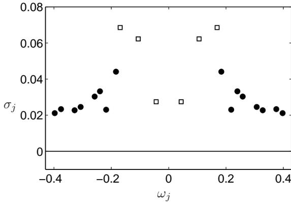
FIGURE 7. The linear spectrum of the jet in crossflow at  $R = 3$ . The eigenvalues marked with squares correspond to anti-symmetric eigenmodes, whereas black circles correspond to symmetric eigenmodes.
