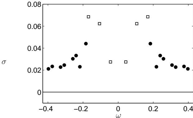
FIGURE 2.2. The linear spectrum of the jet in crossflow at  $R = 3$ . The eigenvalues marked with open squares correspond to anti-symmetric eigenmodes, whereas black circles correspond to symmetric eigenmodes.
