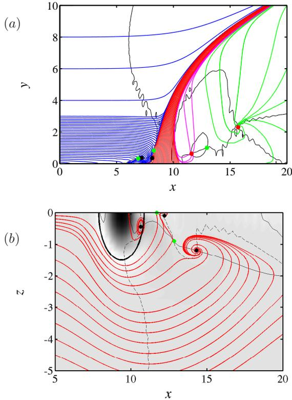
FIGURE 5. Two-dimensional cuts of the steady flow, (a) in a  $z = 0$  plane and (b) in a wall-parallel plane close to the wall. The solid black lines correspond to zero streamwise velocity  $u = 0$ , the dashed black lines to  $v = 0$ . Saddle points are indicated by green dots; nodes with red dots and foci with black dots. Streamlines are plotted with colored lines. In (b) the background gray shade corresponds to the amplitude of the total velocity  $(u^2 + v^2)^{1/2}$ .
