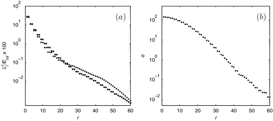
FIGURE 5. (a) The normalized eigenvalues  $\lambda_i^c$  (squares) and  $\lambda_i^o$  (circles) associated with controllable modes and observable modes respectively. (b) The Hankel singular values  $\sigma_i$  corresponding to the balanced modes.
