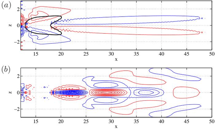
FIGURE 2.6. Wall-normal vorticity at  $y = 1$  for the steady baseflow (a) and mode C (b). Contour levels are  $0.1, 0.2, \dots, 1.0 \cdot \omega_{y,\max}$ , red is positive, blue negative. Inside the region marked by solid black line there is a backflow. The small-scale wiggles are numerical artifacts. Only a portion of the  $xz$ -plane is shown
