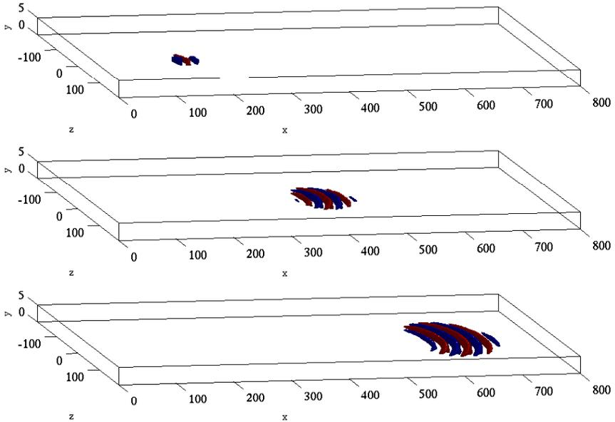
FIGURE 2. Impulse response to an optimal initial disturbance in  $\mathbf{B}_1$  at  $t = 400, 1008, 1600$ . The disturbance is represented by the iso-surfaces of the streamwise component, where the red and blue colours represent positive and negative velocities, respectively.
