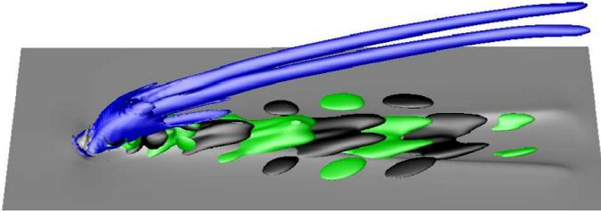
FIGURE 8. Isocontours of the spanwise velocity component pertaining to the low-frequency mode  $((\lambda_r, \lambda_i) = (0.027, 0.27))$ , marked  $W_1$  in the spectrum (figure 5) are shown in green (negative  $w$ ) and black (positive  $w$ ). Note that here only the structures near the wall are shown, which are approximately one order of magnitude smaller in amplitude than the structures on the CVP. The base flow is again in blue ( $\lambda_2$ ) and gray ( $u$ -velocity).
