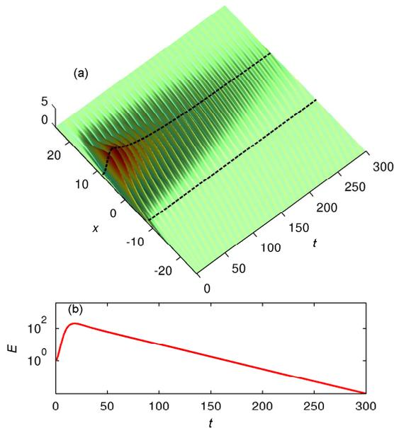
FIGURE 5. (a) Linear transient growth of a perturbation in space and time: an optimal initial perturbation grows as it enters the unstable domain at branch I at  $x = -8.2$  until it reaches branch II at  $x = 8.2$ . The two dashed lines depict branch I and II. (b) The corresponding optimal energy growth of the convectively unstable flow in (a).
