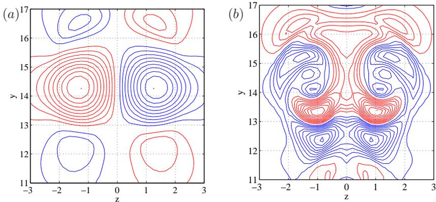
FIGURE 2.4. Streamwise vorticity at  $x = 40$  for the steady baseflow (a) and mode A (b). Contour levels are  $0.1, 0.2, \dots, 1.0 \cdot \omega_{x,\max}$ , red is positive, blue negative. Only a portion of the  $zy$ -plane is shown.
