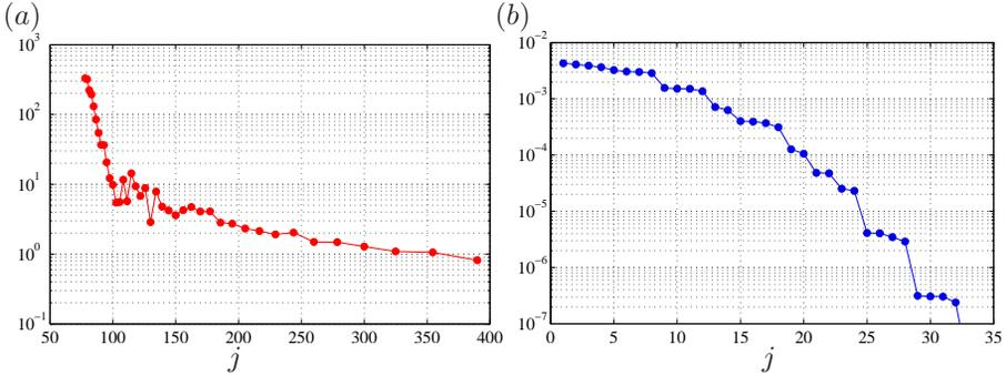
FIGURE 4.2. The average residuals, given by equation (4.13) as function of the number of snapshots included in  $\mathbf{X}_r$  are shown in (a). The magnitude  $a_j$  of the 32 first Ritz values computed for  $r = 390$  is shown in (b).
