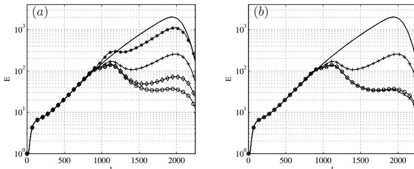
FIGURE 10. Kinetic energy as function of time. In (a) and (b), the solid line shows the energy of  $\mathbf{B}_1$ . In (a) case D ( $-\star-$ ), E ( $-+-$ ), F ( $-\diamond-$ ) and A ( $-\circ-$ ) are characterized by 3, 5, 7 and 9 actuators respectively. In (b) the curves correspond to case E ( $-+-$ ), G ( $-\times-$ ) and A ( $-\circ-$ ) with 5, 5 and 9 sensors, respectively.
