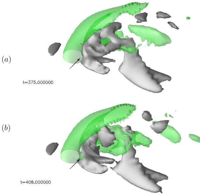
FIGURE 6. Instantaneous visualization of the region close to the jet orifice at  $t = 375$  and  $t = 408$ . Green isocontours correspond to  $v = 0.1$  and grey contours to  $u = -0.1$ . The arrows indicate the location of the low-frequency spanwise oscillation of the separation region.
