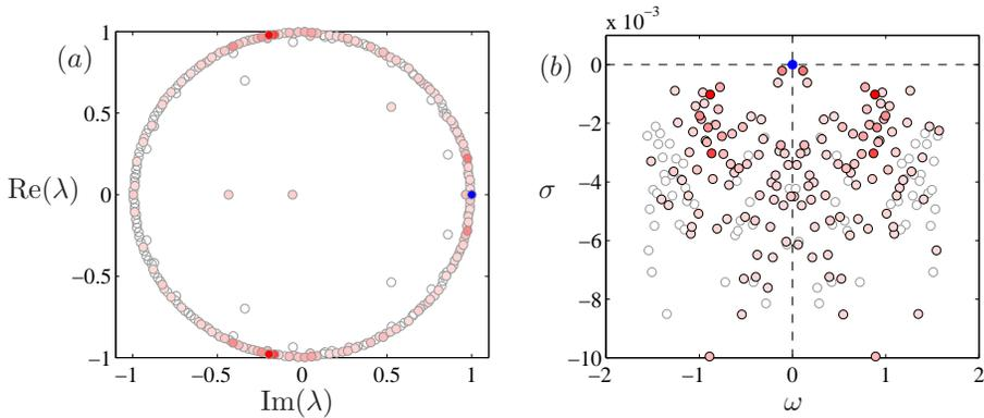
FIGURE 2.7. Time-discrete (a) and time-continuous (b) Koopman spectra of the JCF. The Koopman eigenvalue  $\lambda_0$  is shown with a blue symbol, while the other eigenvalues vary smoothly in color from red (high magnitudes) to white, depending on the magnitude  $\varphi_j$  of the corresponding Koopman mode.
