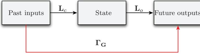
FIGURE 3.5. The controllability operator  $\mathbf{L}_c$  relates past inputs to the present state, while the observability mapping  $\mathbf{L}_o$  relates the present state to the future outputs. Their combined action is expressed by the Hankel operator  $\mathbf{\Gamma}_G$ .
