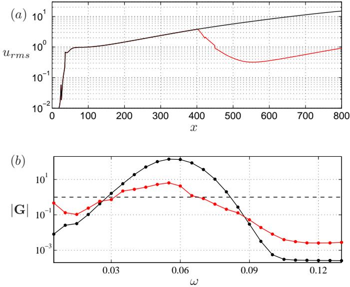
FIGURE 3.9. (a) The streamwise rms-values of the uncontrolled system (blacks), and the closed-loop (red) as a function of the streamwise direction  $x$ . (b) Comparison of the frequency response from disturbances to objective function of uncontrolled (black) and the closed-loop system (red).
