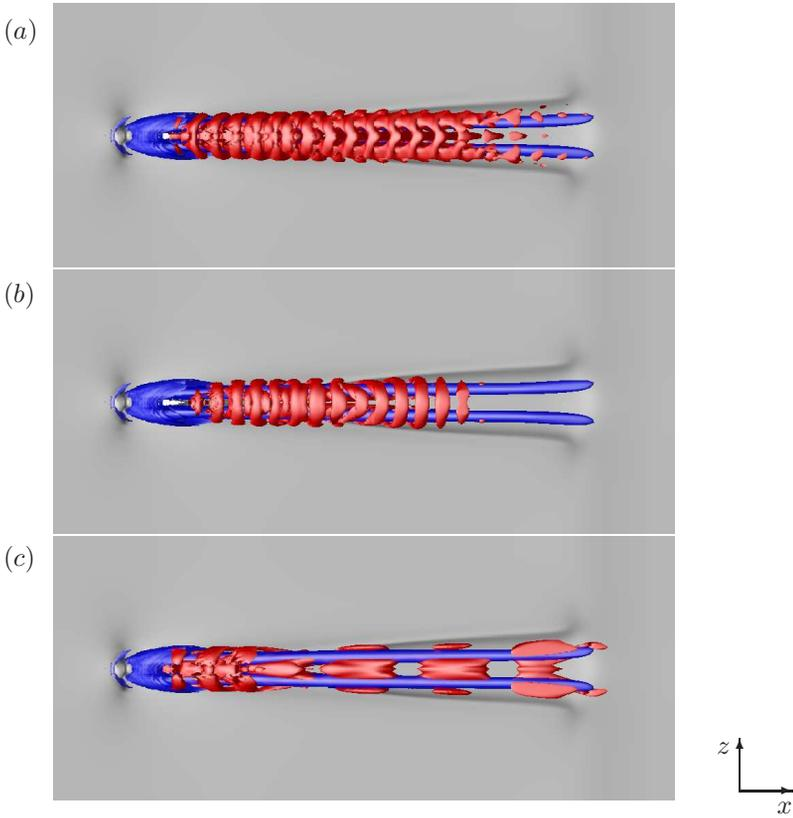
FIGURE 2.3. Linear global eigenmodes A, B and C of the jet in crossflow shown from top view. The red contour levels represent the  $\lambda_2$  criterion, whereas the baseflow is shown in blue ( $\lambda_2$ ) and gray ( $u$ ). The modes are complex and shown at one phase only.
