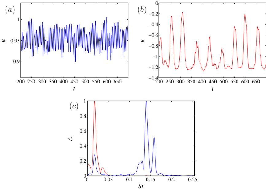
FIGURE 3. (a),(b) Time signals and (c) power spectrum of two probes in the flow. The red line corresponds to a probe located in the separated region downstream of the jet,  $(x, y, z) = (10.7, 1, 0)$ , the blue line corresponds to a probe in the shear layer,  $(x, y, z) = (12, 6, 2)$ .
