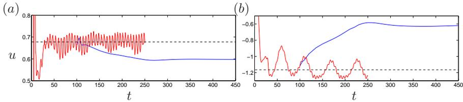
FIGURE 3. (a) and (b) show time signals corresponding to the (streamwise)  $u$ -component of two probes in the flow field (see text). The red line represents the unsteady flow, whereas the blue line corresponds to the simulation stabilized by SFD which is active for  $t > 100$ . The dashed lines indicate the time-averaged values of the DNS simulation.
