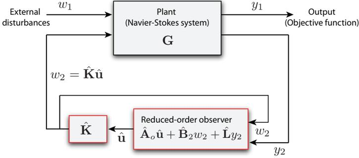
FIGURE 3.8. Sketch of the closed-loop system  $\mathbf{G}_c$ . The controller (red borders) of order  $r$  consists of an observer and feedback gain  $\hat{\mathbf{K}}$  that forces the plant  $\mathbf{G}$  of size  $n$  with the control signal  $w_2$  based on the noisy measurements  $y_2$  so that the effect of  $w_1$  on the output signal  $y_1$  is minimized. The observer is governed by  $\hat{\mathbf{A}}_o \hat{\mathbf{u}} + \hat{\mathbf{B}}_2 w_2 + \hat{\mathbf{L}} y_2$ .
