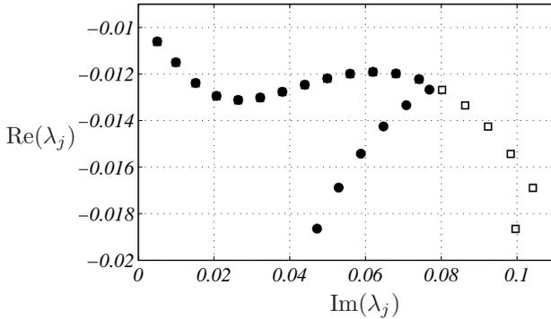
FIGURE 2. Spectrum of of the 2D Blasius flow computed using the timestepping technique with  $\Delta t = 30$  (squares) and  $\Delta t = 40$  (circles). The high-frequency eigenvalues of the latter computation are mapped/aliased into the low-frequency domain.
