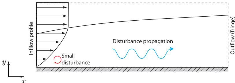
FIGURE 1.1. Sketch of a numerical experiment of the evolution of a wavepacket disturbance in a flat-plate boundary layer. The Reynolds number at the computational inlet is  $Re_x \approx 3 \times 10^5$  and the computational outlet it is  $Re_x \approx 1 \times 10^6$ . The numerical parameters are given in table 4.2 (case 3D-NLIN-BL) in section 4.4 of this thesis.
