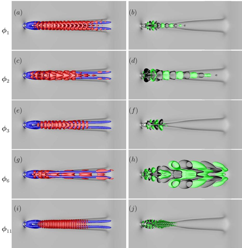
FIGURE 8. Top view of 5 eigenmodes. Left column: contour levels of the  $\lambda_2$  criterion, whereas the baseflow is shown in blue ( $\lambda_2$ ) and gray ( $u$ ). Right column: the structure of the modes near the wall with positive (black) and negative (green) contours of the  $w$  component. The growth rate of the modes decrease from top to bottom. Modes shown on row 1,2 and 4 are anti-symmetric whereas row 3 and 5 show high-frequency symmetric modes.
