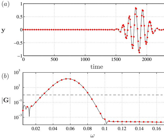
FIGURE 3.4. Impulse (a) and frequency response (b) of the flat-plate boundary layer. The black lines show responses from DNS computations ( $n \approx 10^5$ ). The red symbols show the responses from the reduced-order model ( $r = 60$ ).
