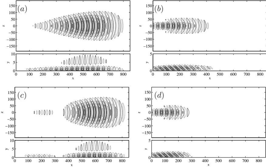
FIGURE 4. Left column: Streamwise component of the leading balanced mode  $\phi_1$  (a) and the third balanced order mode  $\phi_3$  (c). Right column: corresponding adjoint modes  $\psi_1$  (b) and  $\psi_3$  (d). Positive velocity is represented in black, while negative one is in gray.
