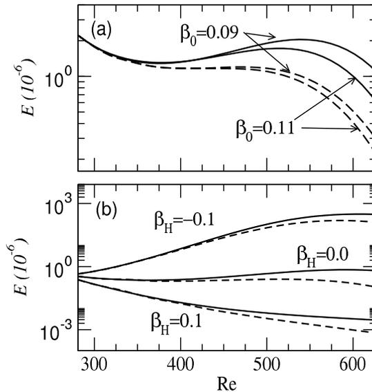
FIGURE 5. (a) The downstream development of oblique waves ( $F = 131.6$ ) in the absence (solid) and the presence (dashed) of streaks. (b) The downstream development of a TS-wave ( $F = 131.6$ ) in the absence (solid) and the presence (dashed) of streaks in boundary layer with adverse, zero and favorable pressure gradient.
