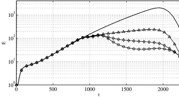
FIGURE 8. Disturbance energy as function of time. The solid line represents the energy growth of the disturbance  $\mathbf{B}_1$ . Also shown are the closed-loop configurations for three different control penalties: a cheap case ( $-\circ-$ ), an intermediate case ( $-\diamond-$ ) and an expensive case ( $-\triangle-$ ).
