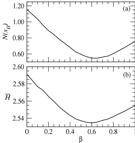
FIGURE 3. (a) The N-factor at branch II of the TS-wave ( $F = 131.6$ ) as a function of the spanwise wavenumber of streaks. The maximum amplitudes of the streaks have been fixed at  $A_s^* = 10\%$ . (b) The averaged shape factor  $\bar{H}$  as a function of the same set of streaks as in (a).
