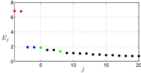
FIGURE 11. The energy  $E_j = \gamma_j / \sum_i \gamma_i \times 100$  of the POD modes with  $j = 1, \dots, 20$ . The POD modes and coefficients corresponding to the eigenvalues depicted in color are shown in figures 12 and 13, respectively. Red: antisymmetric high-frequency mode, blue: symmetric high-frequency mode, green: low-frequency mode.
