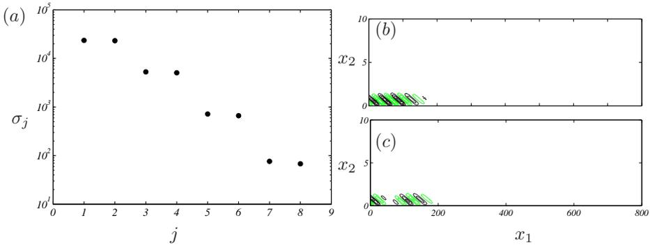
FIGURE 4. (a) Eigenvalues of  $\mathbf{T}^*\mathbf{T}$  computed using the forward and adjoint time stepper with  $t = 1800$ . (b) Streamwise velocity component of the optimal disturbance corresponding the largest eigenvalue in (a). (c) Streamwise velocity component of a suboptimal, corresponding to the third largest eigenvalue in (a).
