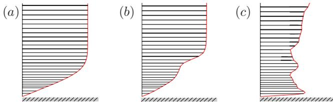
FIGURE 1.3. Velocity profiles of the streamwise component ( $u$ ) as a function of the wall-normal distance from the plate ( $y$ ). The profiles (a), (b) and (c) correspond to the snapshots (a-c) in figure 1.2 and are extracted approximately in the center of the disturbance.
