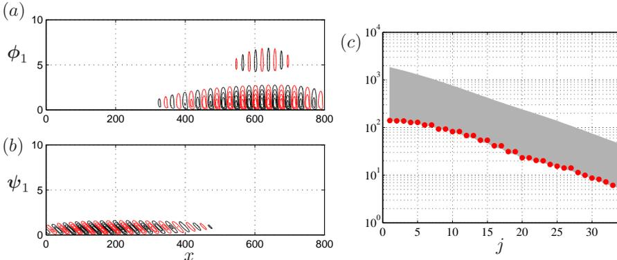
FIGURE 3.7. Left: The streamwise velocity component (positive in red and negative in black) of first balanced mode  $\phi_1$  and its associated adjoint mode  $\psi_1$ . Right: The  $\infty$ -norm model reduction error. The upper and lower theoretical bounds (equation 3.18) are depicted with a gray region and the actual model reduction error is shown with red symbols.
