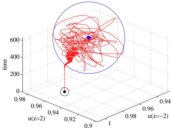
FIGURE 2.1. The streamwise velocity at  $(x, y, z) = (12, 6, \pm 2)$  is plotted as function of time. The black circle marks the region where the flow behavior is linear, whereas the blue circle marks the nonlinear flow dynamics. The figure shows the entire linear-transient-nonlinear development.
