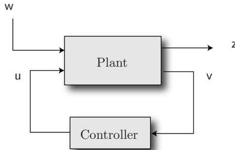
FIGURE 13. The closed-loop system. The plant represent the input–output system given by equation (11) subject to external disturbances  $w$ . The controller of order 50 forces the Navier–Stokes equations with the input signal  $u$  based on the noisy measurements  $v$  so that the effect of  $w$  on the output signal  $z$  is minimized.
