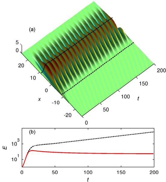
FIGURE 4. (a) The spatio-temporal evolution of a disturbance in a globally unstable flow. The disturbance grows exponentially until the cubic nonlinear term  $-|q|^2q$  (see Chomaz *et al.* 1990; Chomaz 2005, for details of the nonlinear Ginzburg-Landau equation) causes the disturbance to saturate and oscillate. (b) The energy that corresponds to the evolution in (a) is shown in red, and the linear exponential growth for the linear Ginzburg-Landau equation is shown in dashed black.
