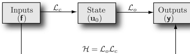
FIGURE 2. The operators used to examine the system input–output behavior. The controllability operator  $\mathcal{L}_c$  relates past inputs to the present state, while the observability mapping  $\mathcal{L}_o$  relates the present state to the future outputs. Their combined action is expressed by the Hankel operator  $\mathcal{H}$ .
