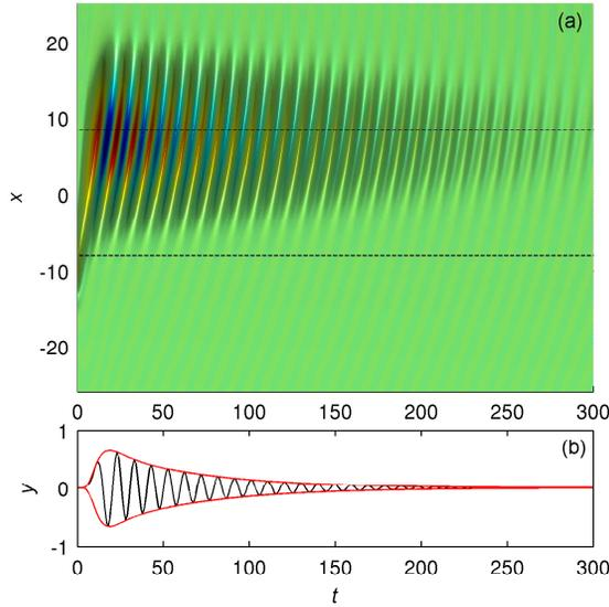
FIGURE 10. Impulse response of the Ginzburg-Landau equation: (a) The state response to an impulse introduced at  $t = 0$  and  $x_w = -11$ . (b) The impulse response at branch II. The convective character of the instability is evident: a wavepacket grows as it enters the unstable domain, but is gradually convected away from this domain before it begins to decay.
