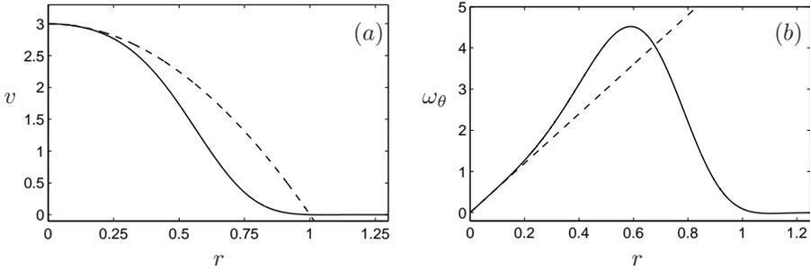
FIGURE 1. The wall-normal velocity  $v$  (a) and azimuthal vorticity  $\omega_\theta = -\partial_r v$  (b) of the imposed jet profile in the present study given by equation (1) is shown with solid black lines and the standard Poiseuille parabolic profile is shown with dashed lines. Note that the streamwise  $u$  and spanwise  $w$  velocities are assumed to be zero everywhere at  $y = 0$ .
