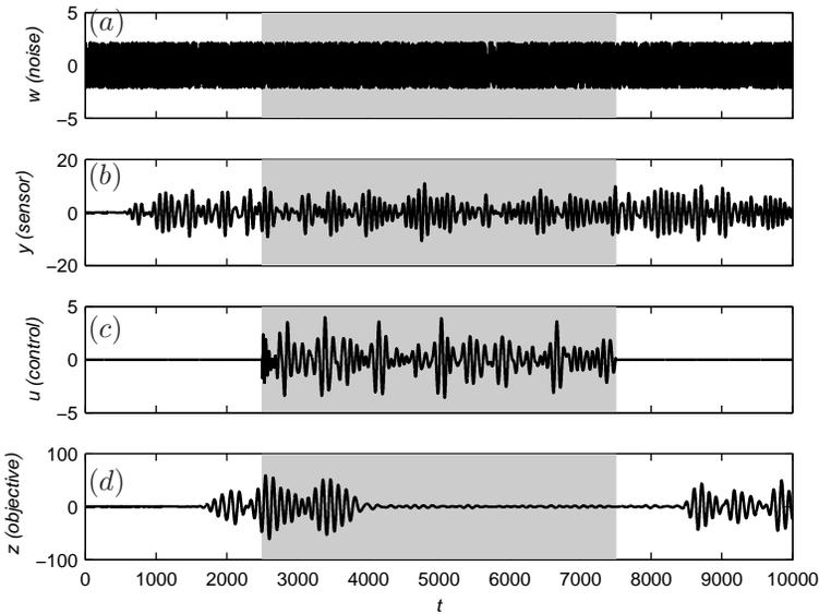
FIGURE 14. Input and output signals of the closed-loop system. The the random forcing  $w$  (a), measurements signal  $v$  (b), control signal  $u$  (c) and the objective function  $z$  (d) is shown. The cheap controller is active between  $t \in [2500, 7500]$  marked with the gray area.
