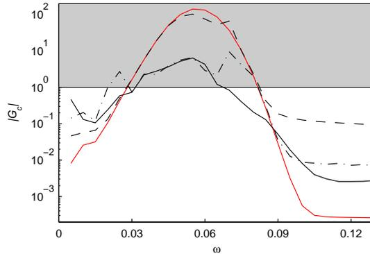
FIGURE 16. Comparison of the frequency response from disturbances to objective function ( $\mathcal{B}_1 \rightarrow \mathcal{C}_1$ ) of open-loop (red) and three closed-loop systems. The cheap, intermediate and expensive controllers are represented by the solid black, dashed-dotted and dashed lines respectively. The infinity norm of the open loop is  $\|G\|_\infty$  is 140.7, whereas for the closed-loop systems  $\|G_c\|_\infty$  it is 6.4 (cheap), 9.4 (intermediate) and 101.9 (expensive).
