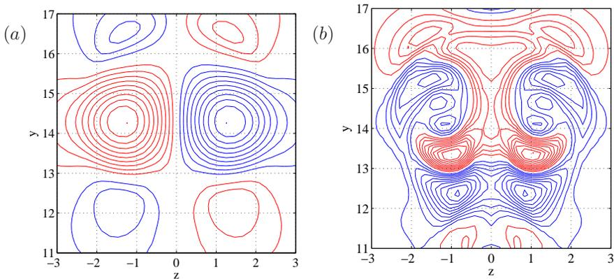
FIGURE 10. Streamwise vorticity at  $x = 40$  for the steady base flow (a) and the most unstable mode (b). Contour levels are  $0.1, 0.2, \dots, 1.0 \cdot \omega_{z,\max}$ , red is positive, blue negative.
