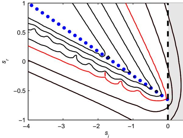
FIGURE 11. Input-output pseudospectra where the black transfer function contour levels are  $\{10^0, 10^1, 10^3, 10^4, 10^5, 10^6\}$ . The red contour (with level 208) represents the largest contour value that crosses the imaginary axis. The blue symbols indicate the eigenvalues of  $A$ .
