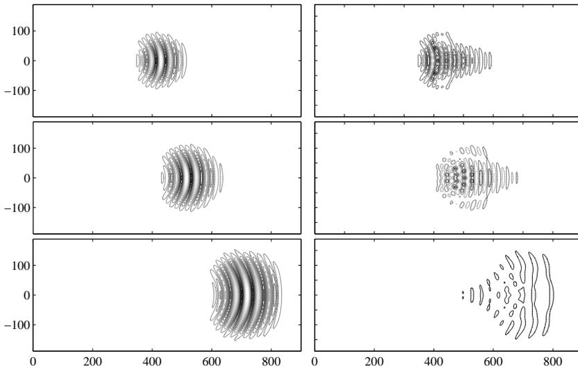
FIGURE 9. Impulse response to an optimal disturbance at  $t = 1000, 1250, 1750$  without control (left column) and with control (right column). The iso-contours of the streamwise component are shown in the  $xz$ -plane at  $y = 2$ .
