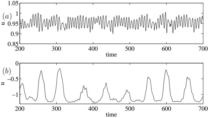
FIGURE 1.7. Time signals of two probes measuring the streamwise velocity  $u$  component at a single point in the flow. In (a) the probe is placed in the shear layer and in (b) near the separated region downstream of the jet near the wall.
