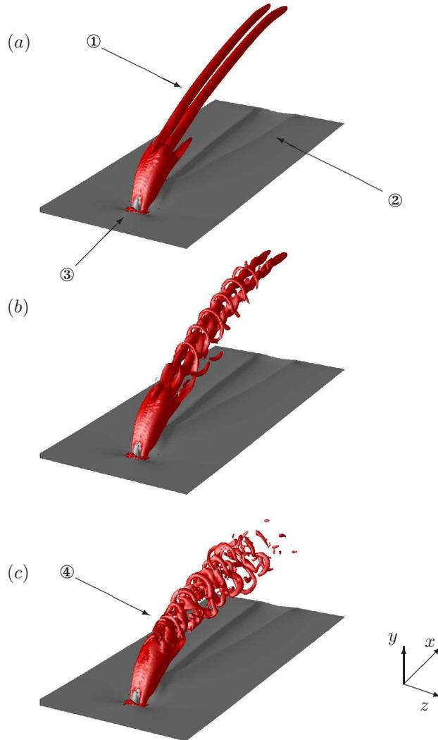
FIGURE 1.6. Three instantaneous snapshots of the steady-unsteady transition at  $t = 0, 300$  and  $t = 500$  are shown in (a), (b) and (c) respectively. Red contour levels represent the  $\lambda_2 = -0.09$  and the gray contour levels represent the streamwise velocity  $u = 0.2$ . See text for explanations of labels ①-④.
