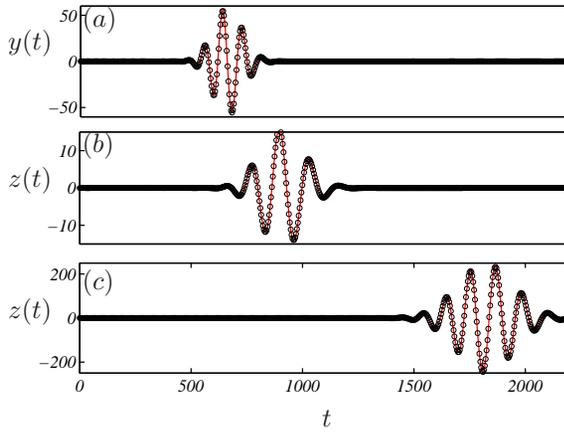
FIGURE 10. The impulse response from  $B_1 \rightarrow C_2$  (a),  $B_2 \rightarrow C_1$  (b) and  $B_1 \rightarrow C_1$  (c). The black solid line represents direct numerical simulations with  $10^5$  degrees of freedom and the red dashed line the balanced reduced-model with 70 degrees of freedom.
