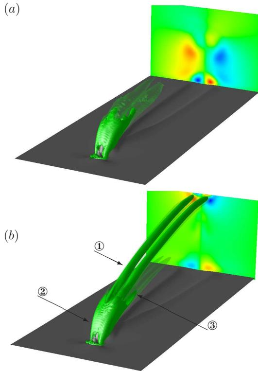
FIGURE 2. (a) Mean flow and (b) steady flow obtained by SFD visualized by iso-contours of  $\lambda_2 = -0.09$  (solid green),  $\lambda_2 = -0.01$  (opaque green) and  $u = 0.2$  (grey) close to the wall. The vertical plane towards the end of the domain is color-coded according to the spanwise velocity component. The numbered labels are discussed in the text.
