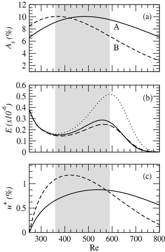
FIGURE 2. (a) Evolution of amplitudes of two streaks with  $\beta = 0.45$  (solid) and  $\beta = 0.65$  (dashed). (b) TS wave with  $F = 131.6$  in absence (dotted) and presence (dashed, solid) of streaks. (c) The maximum value of the mean flow distortion caused by the streaks.
