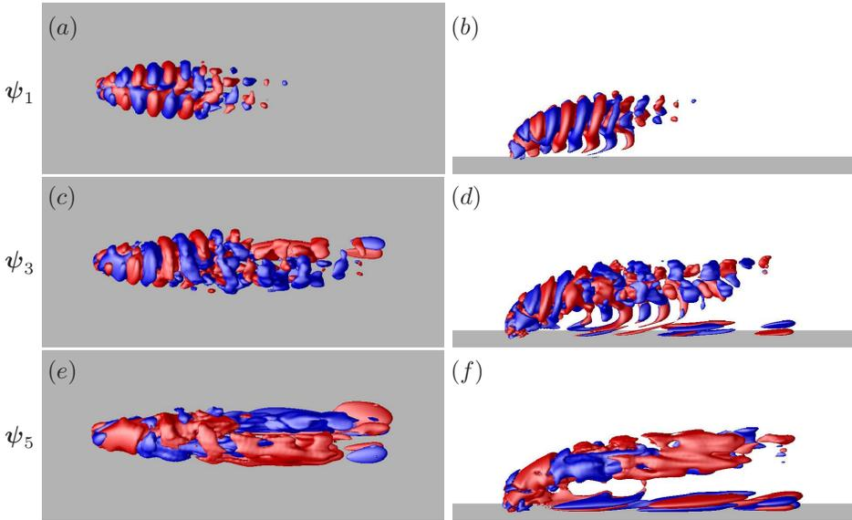
FIGURE 12. Positive (red) and negative (blue) isocontours of the  $u$ -velocity of 3 POD modes from top view and side view. The first row corresponds to the modes marked with red circles; the second row to blue circles and the third row to green circles in figure 11.
