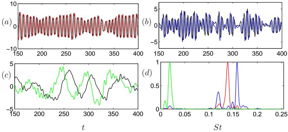
FIGURE 13. The temporal behavior of POD modes are show in terms of the POD coefficients. (a) POD coefficients of the first pair, (b) second pair and (c) third pair of modes. The power spectrum of the signals in (a,b,c) is shown with the same color.
