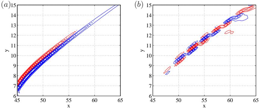
FIGURE 2.5. Spanwise vorticity at  $z = 0$  for the steady baseflow (a) and the mode B (b). Contour levels are  $0.1, 0.2, \dots, 1.0 \cdot \omega_{z,\max}$ , red is positive, blue negative. Only a portion of the  $xy$ -plane is shown.
