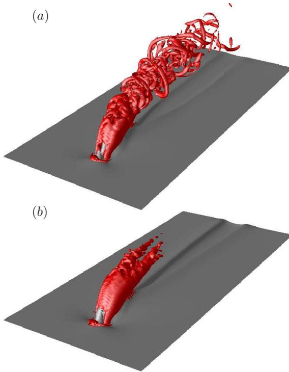
FIGURE 1. (a) Snapshot of the flow field at  $t = 400$ . Red and gray isocontours represent  $\lambda_2 = -0.1$  and  $u = 0.2$  (near the wall) respectively. (b) The same quantities for the time-averaged flow which also is the first Koopman mode.
