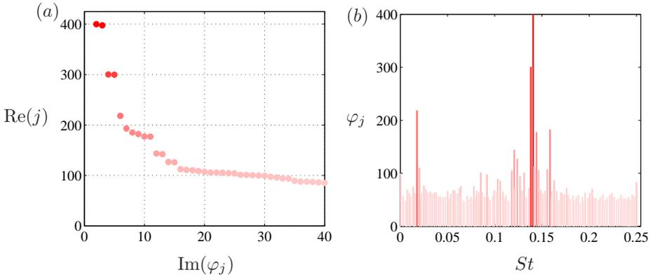
FIGURE 2.8. Left figure: The magnitudes  $\varphi_j$  associated with the Koopman modes  $j = 1, \dots, 40$ . Right figure: The magnitudes  $\varphi_j$  are plotted as a function of the Strouhal number  $St_j$ .
