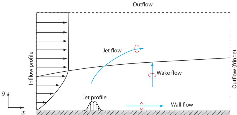
FIGURE 1.5. Sketch of a numerical experiment of the jet in crossflow. The initial fields are the flat-plate boundary layer profile and a parabolic jet profile. The ratio between the jet flow and the crossflow denoted by  $R$ , is three. The numerical parameters are given in table 4.2 (case JCF) in section 4.4.
