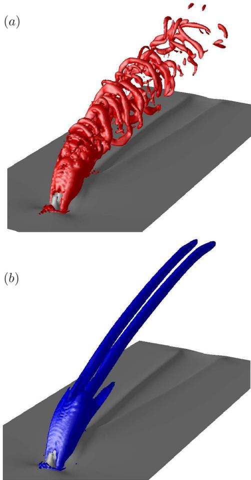
FIGURE 2. (a-b): The red and blue isocontours correspond to vortical structures visualized by the  $\lambda_2$ -criterion (Jeong & Hussain 1995) at a level  $\lambda_2 = -0.09$ . The gray contours depicts the streamwise velocity component  $u = 0.3$  near the flat plate. (a) Snapshot of the unsteady velocity field in a fully-developed state at  $t = 151$ . (b) Converged steady base velocity field.
