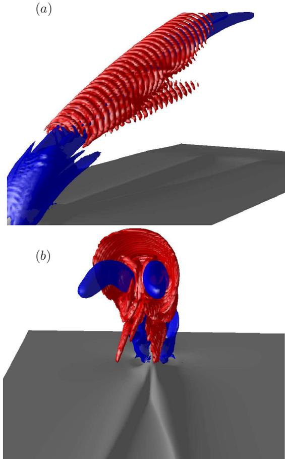
FIGURE 7. The mode with the highest frequency ( $(\lambda_r, \lambda_i) = (0.021, 2.49)$ ) viewed from two different angles, marked with  $S_2$  in figure 5, is shown with red  $\lambda_2$ -isocontours and base flow in blue ( $\lambda_2$ ) and gray ( $u$ -velocity).
