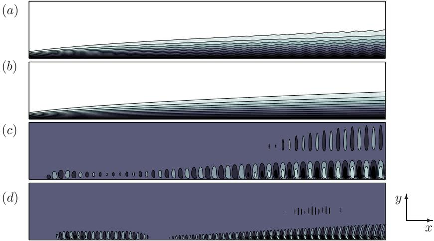
FIGURE 4.3. The streamwise velocity component of a snapshot from the nonlinear simulation at  $t = 85$  (a), the zeroth (b), first (c) and third (d) Koopman modes computed using the algorithm explained in section 4.2.
