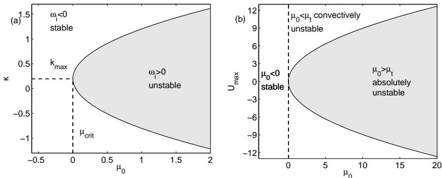
FIGURE 3. (a) The neutral stability curve for the parallel Ginzburg-Landau equation (with  $c_u = 0.2$ ) in the  $(\mu_0, k)$ -plane. (b) The neutral absolute stability curve for the parallel Ginzburg-Landau equation (with  $\gamma = 1 - i$ ) in the  $(\mu_0, U_{max})$ -plane.
