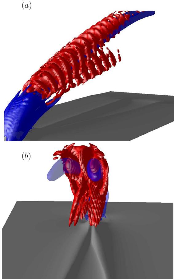
FIGURE 6. The most unstable mode  $((\lambda_r, \lambda_i) = (0.068, 1.06))$  seen from two different angles, marked with  $S_1$  in figure 5 is shown with red  $\lambda_2$ -isocontours. The base flow is shown in blue ( $\lambda_2$ ) and gray ( $u$ -velocity).
