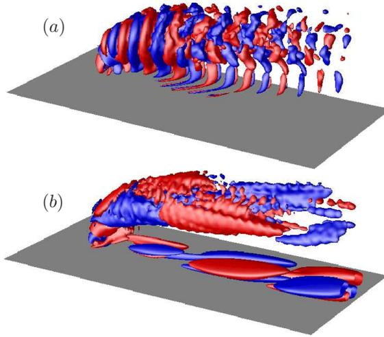
FIGURE 4. Positive (red) and negative (blue) contour levels of the streamwise velocity components of two Koopman modes. The wall is shown in gray. (a) Mode 2, with  $\|\mathbf{v}_2\| = 400$  and  $St_2 = 0.141$ . (b) Mode 6, with  $\|\mathbf{v}_6\| = 218$  and  $St_6 = 0.0175$ .
