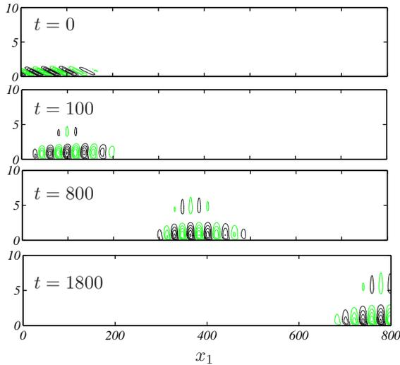
FIGURE 6. Time evolution for streamwise velocity with the combined Orr and TS mechanism, when initiated with the optimal initial condition from  $t = 1800$ . Note that the maximum amplitude is growing from frame to frame following the energy evolution given in figure 5(b).
