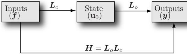
FIGURE 7. The operators used to examine the system input-output behavior. The controllability operator  $L_c$  relates past inputs to the present state, while the observability mapping  $L_o$  relates the present state to the future outputs. Their combined action is expressed by the Hankel operator  $H$ .
