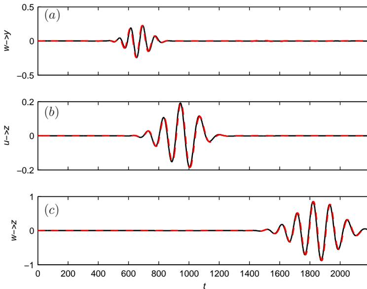
FIGURE 11. The impulse response from  $\mathcal{B}_1 \rightarrow \mathcal{C}_2$  (a),  $\mathcal{B}_2 \rightarrow \mathcal{C}_1$  (b) and  $\mathcal{B}_1 \rightarrow \mathcal{C}_1$  (c). The black solid line represents direct numerical simulations with  $10^5$  degrees of freedom and the red dashed line the balanced reduced-model with 50 degrees of freedom.
