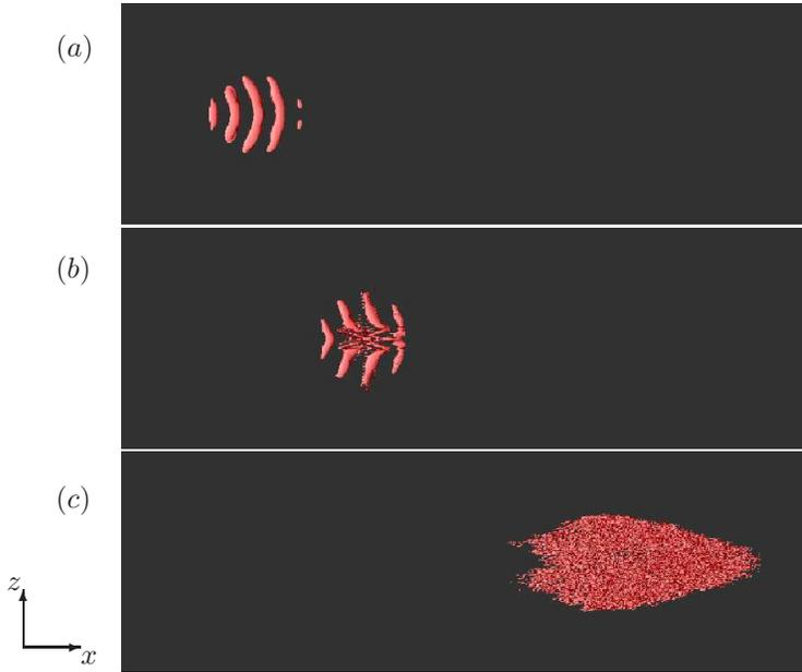
FIGURE 1.2. Snapshots of the disturbance at  $t = 300, 600$  and  $t = 1000$  are shown in (a), (b) and (c) respectively. Red iso-contour levels depict the  $\lambda_2$ -criterion. The plate is shown in black and viewed from top.
