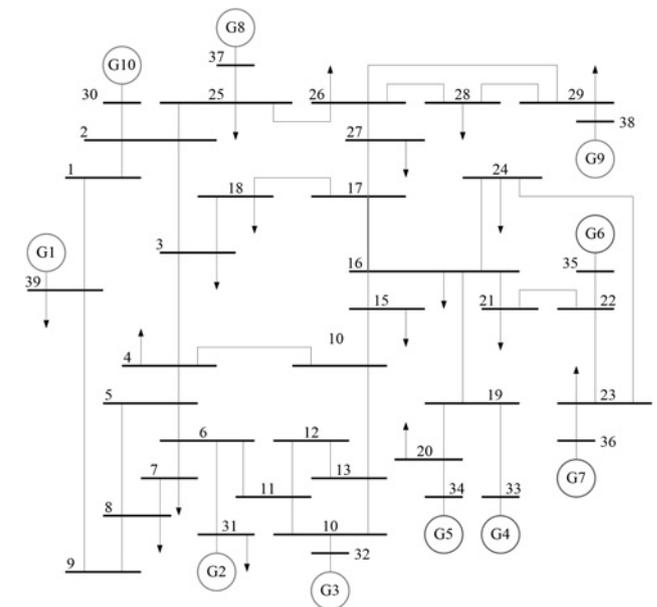
Fig. 2 New England 39-bus test system model
