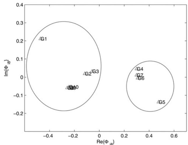
Fig. 6 Coherency identification using the DMD algorithm
