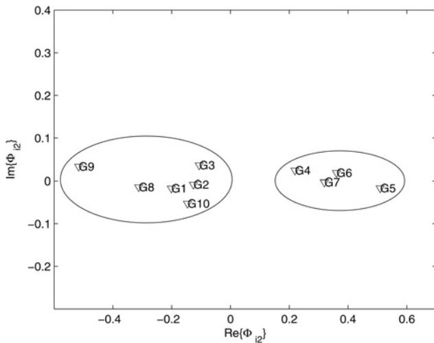
Fig. 7 Coherency identification using the NNR-DMD algorithm
