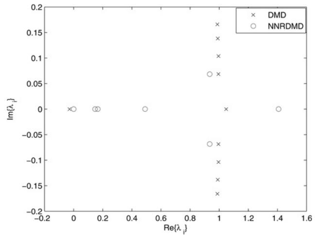
Fig. 5 Eigenvalues  $\lambda_s$  obtained from the DMD and NNR-DMD algorithms
