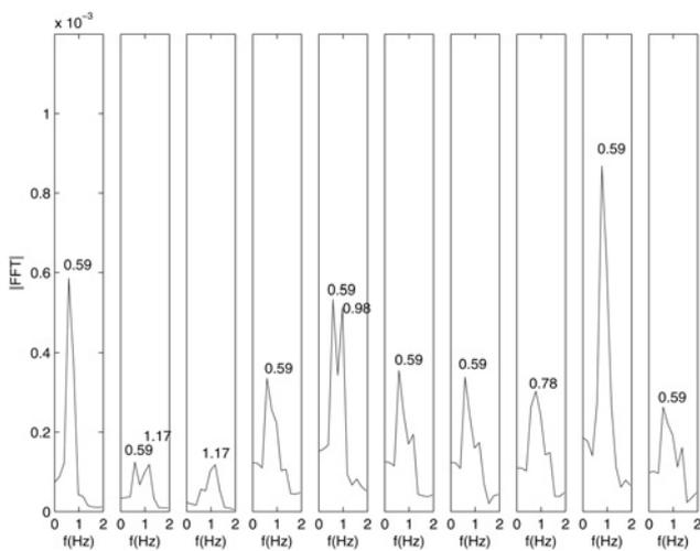
Fig. 4 Spectra analysis results for speed deviations of generators from G1 to G10
