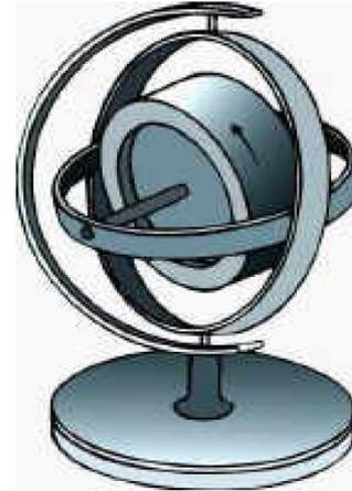
**Mechanical Gyro:** A spinning wheel will resist any change to its angular momentum vector. Maintains constant orientation if in a frictionless gimbal
