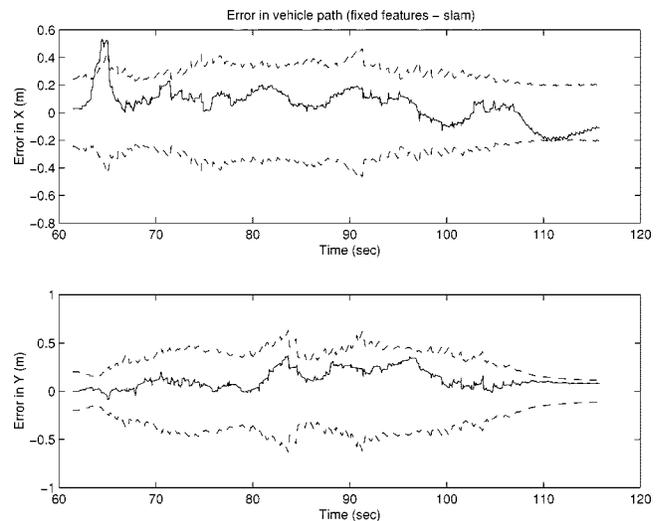
Fig. 8. Actual error in vehicle location estimate in  $x$  and  $y$  (solid line), together with 95% confidence bounds (dotted lines) derived from estimated location errors. The reduction in the estimated location errors around 110 s is due to the vehicle slowing down and stopping.
